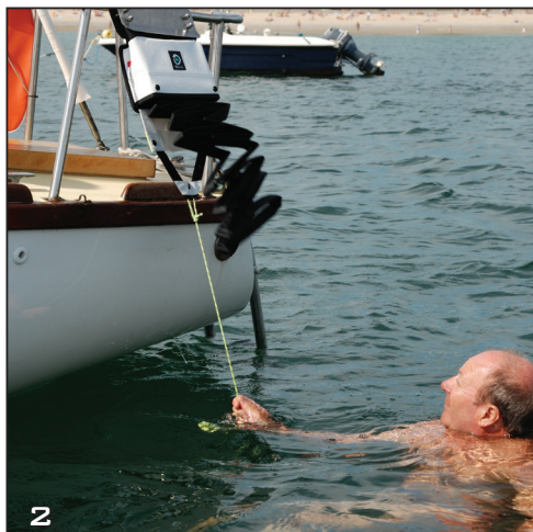
Once the flap is opened, the ladder deploys automatically.
