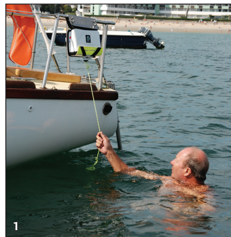
Pull the cord to open the flap of the reboarding ladder case.
