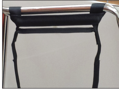
1 Loop the reboarding ladder around the stern rail. The loop of ladder needs to face outboard.
